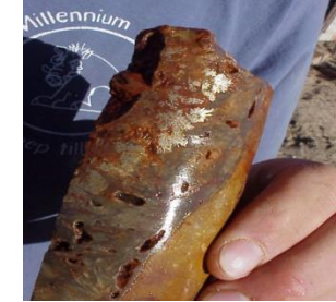
Drill core showing free gold
